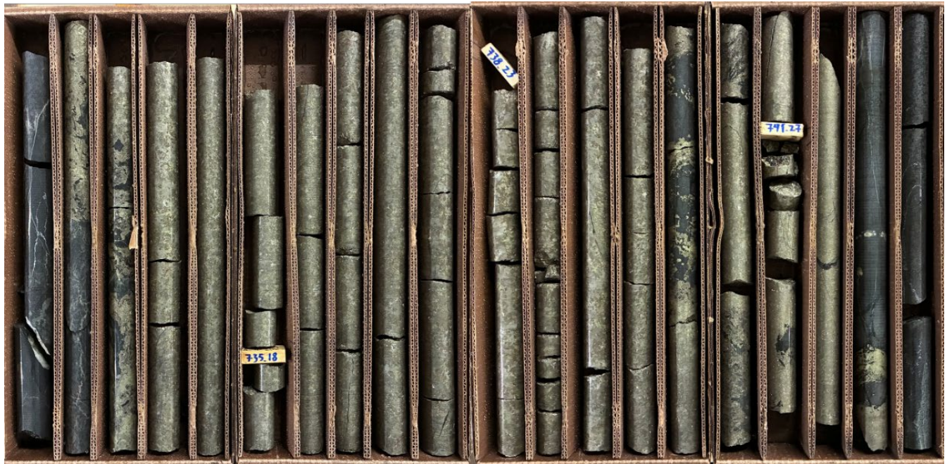
Figure 2: Drill hole 25TK0568A intercepted 8.88 meters grading 9.47% Ni, 14.37% Cu, 0.12% Co, 5.44 g/t Pt+Pd, and 2.86 g/t Au (18.62% NiEq or 36.72% CuEq) starting at 733.15 meters.
